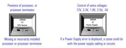
The following diagram shows how the Pre-boot Diagnostics works when it encounters an error.
